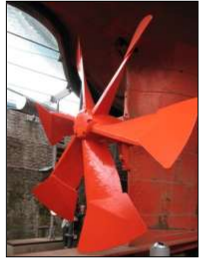
Figure 5. See the people center bottom to gauge the size of the 15-ft (4.6-m) diameter propeller.
