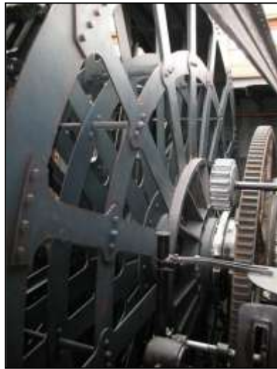
Figure 4. Steam drove four pistons to turn this giant wheel in the Great Britain .
